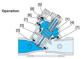
Line Pressure is applied to the Control Chamber [1] through the Internal Strainer [2] and the Orifice [3]. This creates superior closing force that moves the Diaphragm Assembly [4] to a closed position. Opening the Solenoid [5] releases the accumulated pressure from the control chamber, through the Solenoid Seat [6] and the Internal Passage [7] to the downstream, thereby opening the main Valve. The Override Handle [8] enables manual opening.
